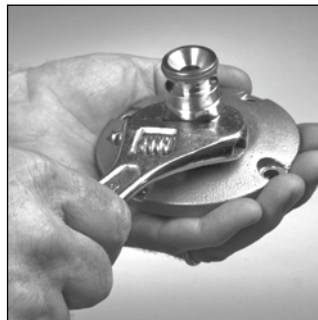
2. Coat coupling threads with a good sealant and tighten coupling onto mounting device*. Re-tighten set screw.
